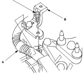
3. Disconnect the 2nd clutch transmission fluid pressure switch connector, and remove the 2nd clutch transmission fluid pressure switch (A).
